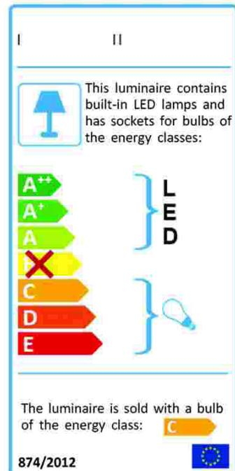
(d) luminaire containing both non-replaceable LED modules and sockets for user-replaceable lamps, with lamps not included:
