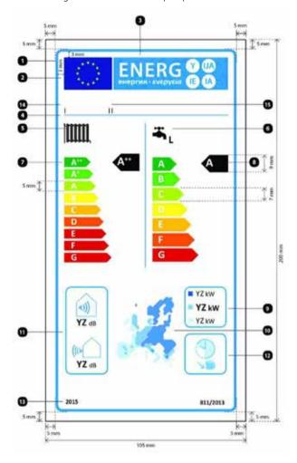
10. The design of the label for heat pump combination heaters shall be the following:
