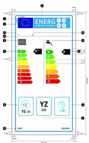
9. The design of the label for boiler combination heaters shall be the following:
