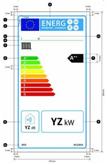
5. The design of the label for boiler space heaters shall be the following:
