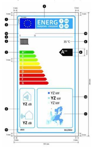
8. The design of the label for low-temperature heat pumps shall be the following:
